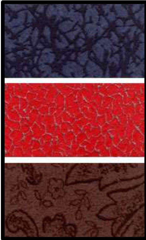
Photographs of products embossed with a Cubitex machine. Engraving with 3D effect on patterns is possible.
